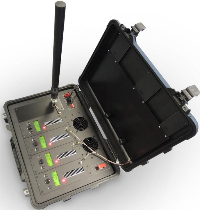
Programmable Jammers help users in the field choose which frequencies they want to block. Requiring no downtime for factory settings, these programmable RF Jammers are flexible and give the user better control over the RF environment.
